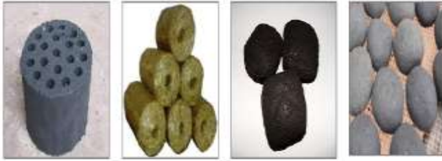
Figure1: From left-right: honey-comb briquette (hydraulic press); non-carbonised straw briquette (piston extruded); carbonised charcoal dust (roller press); hand-made charcoal dust briquettes
