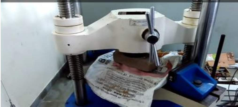
Fig 2.Compression Test on UTM
