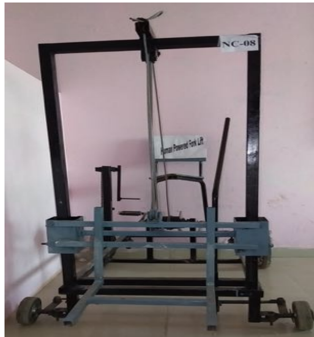
Fig 1 Photographic view of human powered forklift
