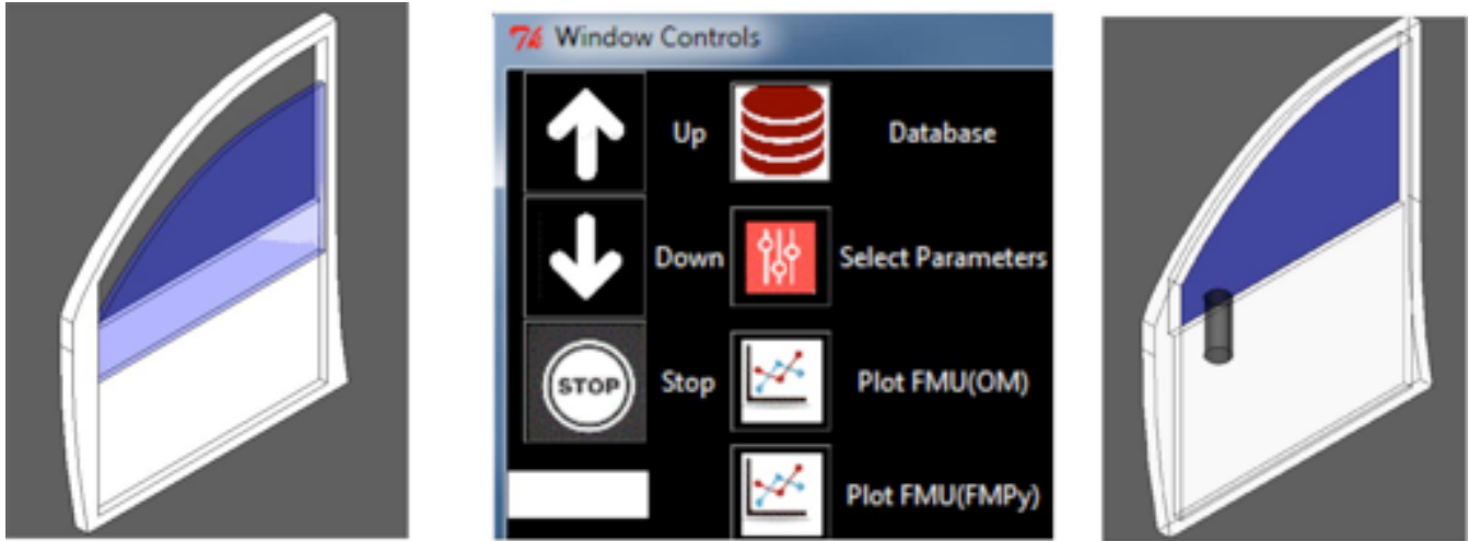
Fig. 6 GUI and CAD models for controlling and visualizing of door lock and power window
