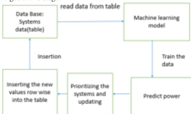
Fig.6. Block diagram showing the prioritization of the predicted powers using EMS algorithm
