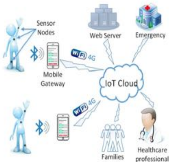
Fig 1. Wireless body area network with IOT connected healthcare platform
