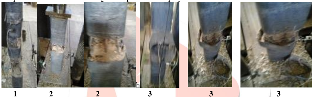
Fig (3) Failure modes of testing columns
