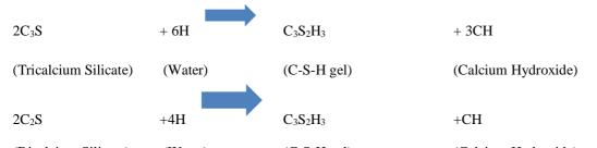
(Dicalcium Silicate) (Water) (C-S-H gel) (Calcium Hydroxide) The hydration products from  $C_3S$  and  $C_2S$  are similar but quantity of calcium hydroxide (lime) released is higher in  $C_3S$  as compared to  $C_2S$ .
