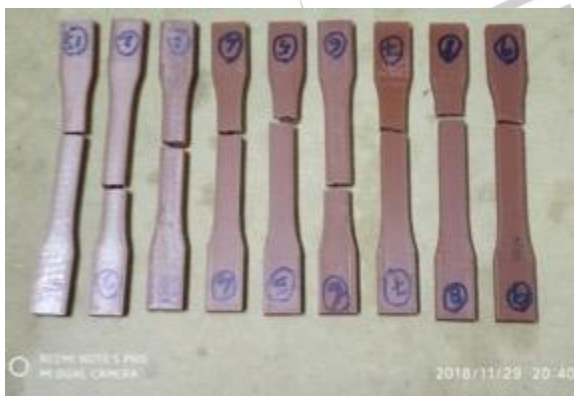
Fig.13. PLA Tensile Test Specimens After Testing
