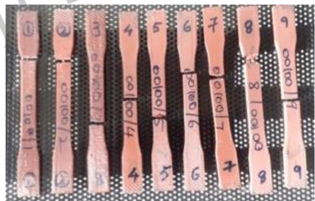
Fig.14. PLA tensile test specimens (Filling Ratio 100%)
