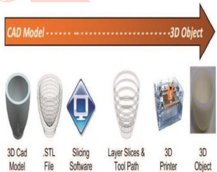
Fig.3 Generalized FDM Process
