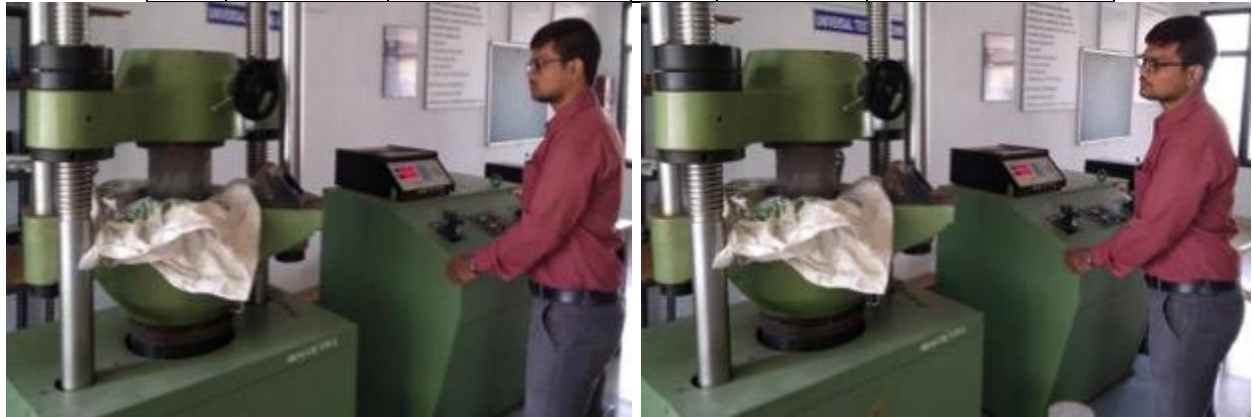
Fig 5. Compressive strength test apparatus
