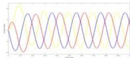
Fig. 21 Three phase source current waveform with SAP filter
