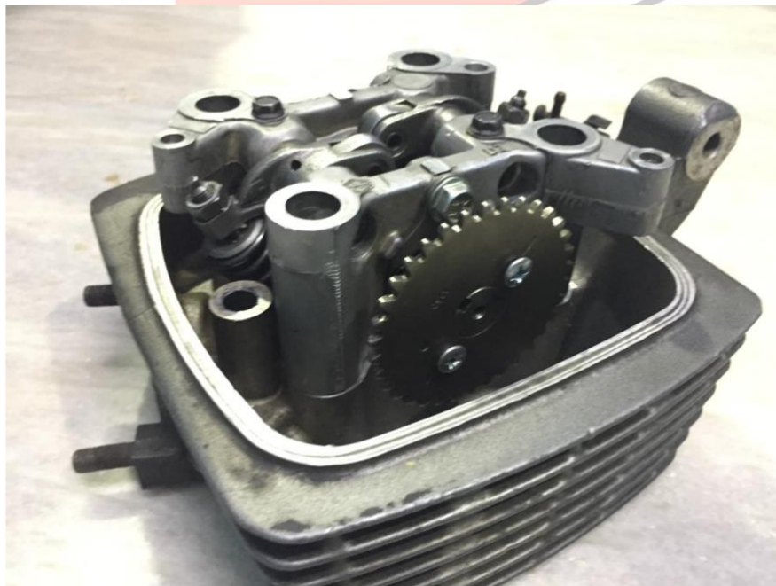
Fig. 11. Engine Head with Cam Assembly
