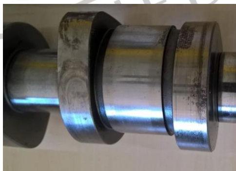
Fig. 3. Cam Lobe Wear cause of Lifter
