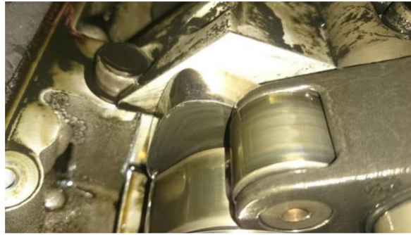
Fig. 4. Lifter Impact on Cam Lobe
