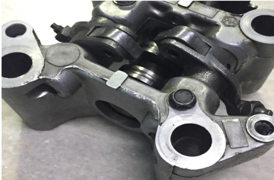
Fig. 12. Assembly of Camshaft with Modified Lifter and Cam
