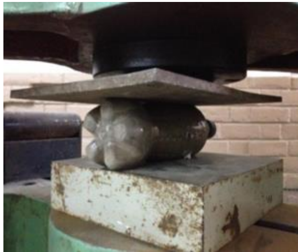
Fig. a.1 -Single bottle under testing machine
