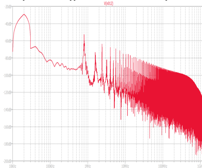
Fig8. SNDR Output of Bootstrapped S/H circuit without Multiplier 90nm_20KHz
