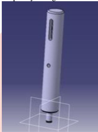
Fig. 3.1: CAD Model of TVS shaft developed in CATIA V5R19.
