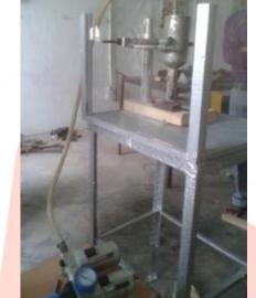
Fig 2 : Fabricated Experimental Setup of Abrasive jet Machining
