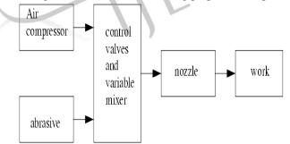
Fig 1: Line Diagram of Abrasive Jet Machining Process
