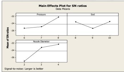
Fig 4: Graphs indicates the Effect of Pressure, Sod, Nozzle diameter on MRR
