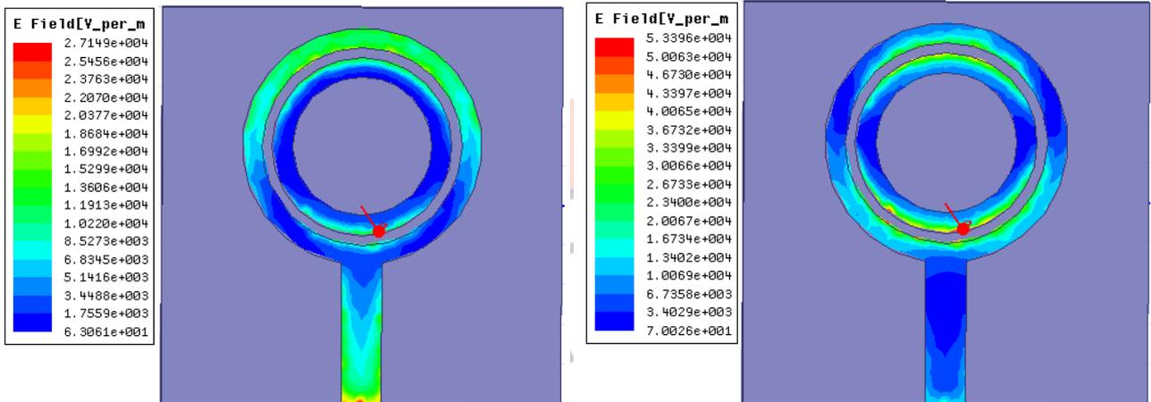
Figure 5: (a) E field pattern at 4.4GHz, (b) E field pattern at 7.3GHz
