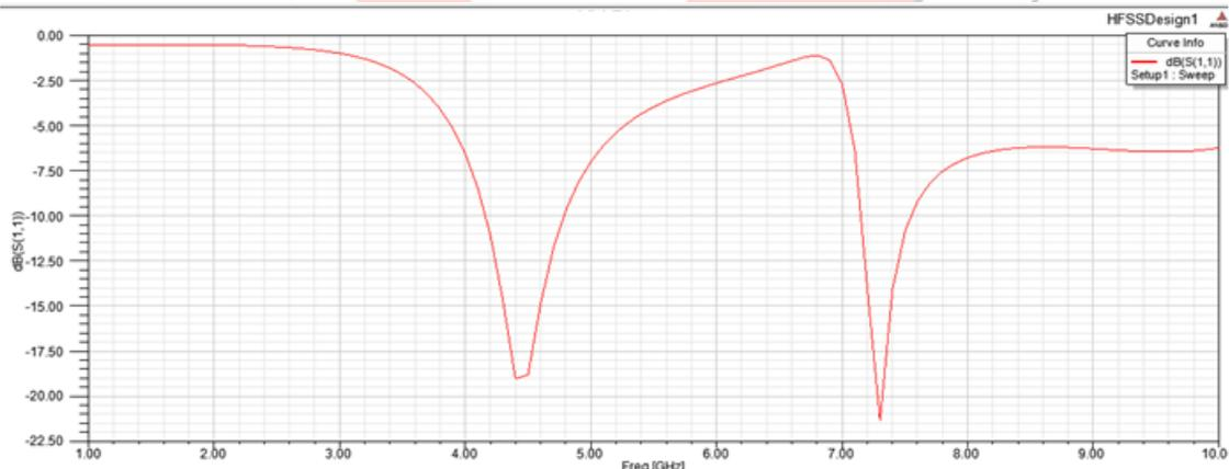
Figure 2: Simulated return loss of the proposed antenna.
