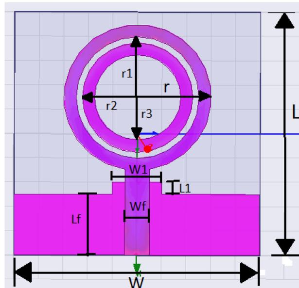
Figure 1: Proposed antenna structure
