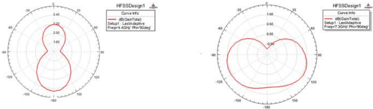
Figure 4: (a) Simulated radiation pattern at 4.4GHz, (b) Simulated radiation pattern at 7.3GHz
