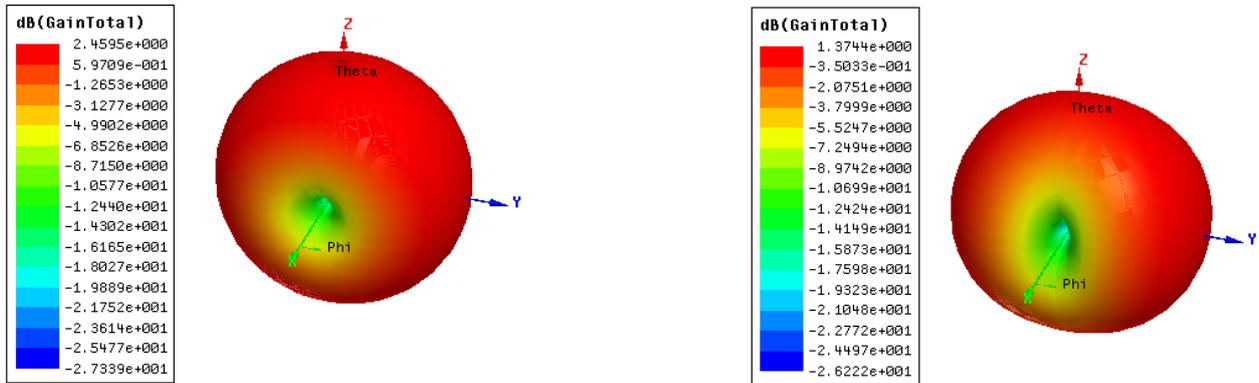
Figure 3: (a) Simulated radiation patterns at 4.4GHz, (b) Simulated radiation patterns at 7.3GHz
