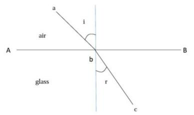
In the diagram, the line AB is the boundary between air and glass, and ab is a ray of light passing from air into glass where it is refracted along the line **bc**. Then whatever may be the value of the angle of incidence (i) the angle of refraction (r) will always be so related to it that
