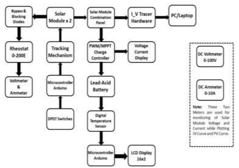
Fig.1 block diagram of solar PV charge controller training system
