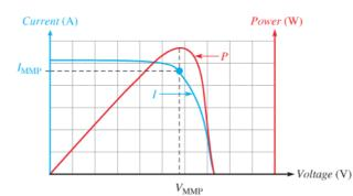
The above figure shows maximum powerpoint. There is only point in the IV\_characteristics of PV module at which power delivered by PV module is maximum. The MPPT and charge controller are two different functions, The developer combined this two function in one electrical circuitry called MPPT charge controller. Advantages:
