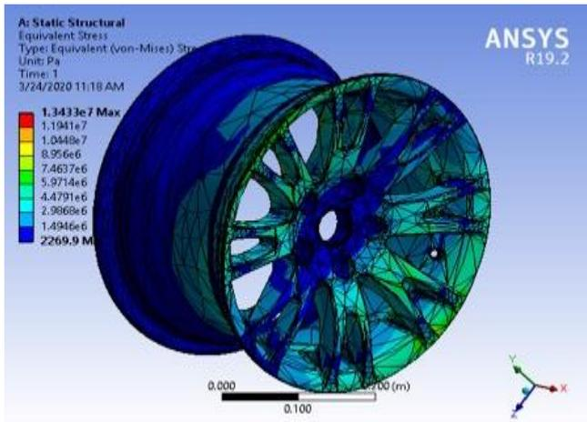
Figure 8. Von-mises stress of Mg-alloy RIM.
