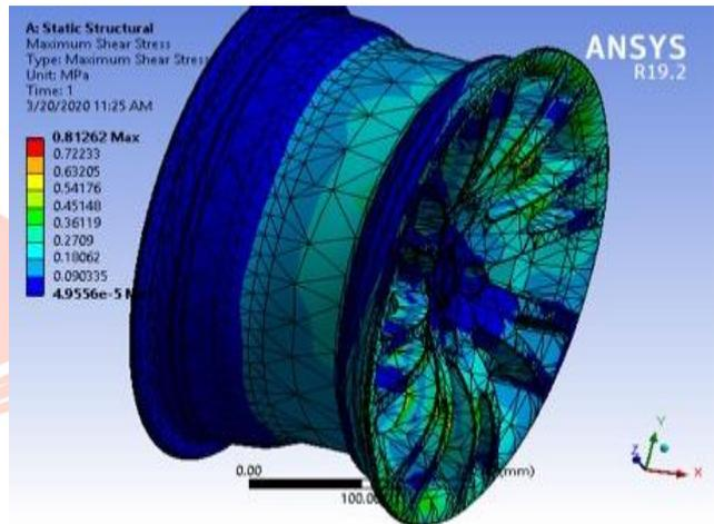
Figure 11. Maximum shear stress of PEEK RIM.
