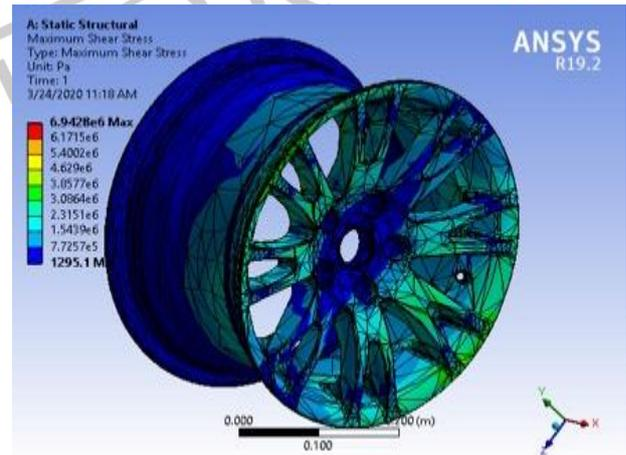
Figure 7. Maximum shear stress of Mg-alloy RIM.
