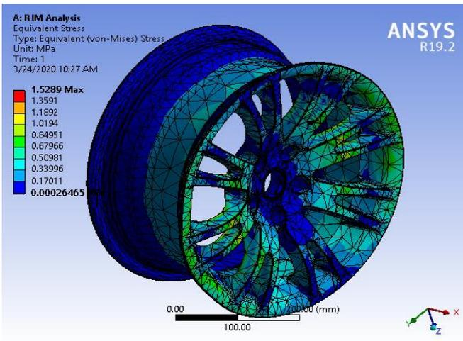
Figure 4. Von-mises stress of Al-alloy RIM.
