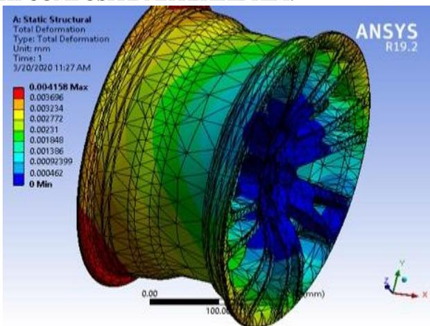
Figure 10. Total deformation of PEEK RIM.
