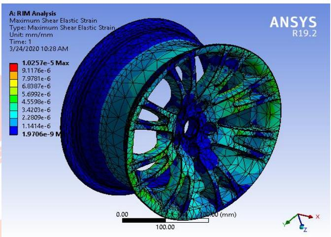
Figure 5. Maximum shear elastic strain of Al-alloy RIM.
