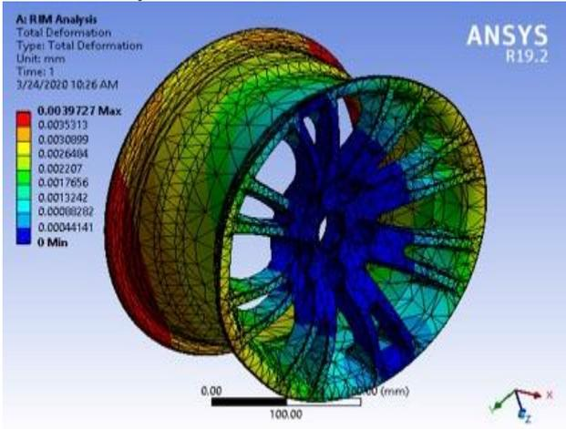
Figure 2. Total deformation of Al-alloy RIM.
