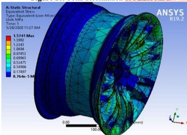
Figure 12. Von-mises stress of PEEK RIM.
