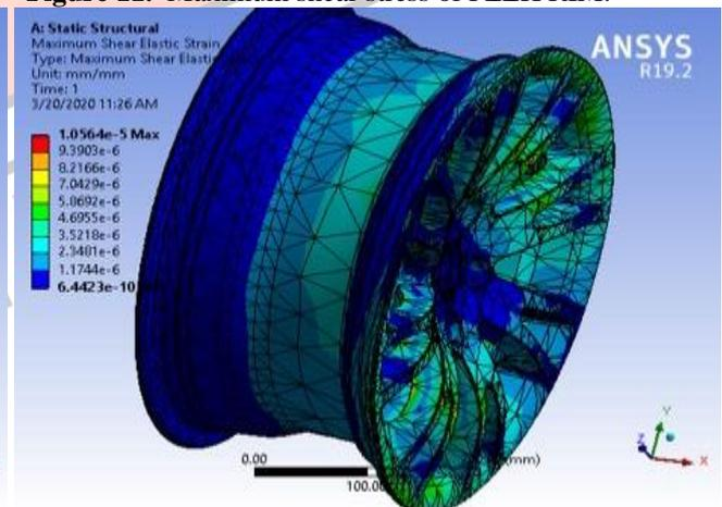
Figure 13. Maximum shear elastic strain of PEEK RIM.
