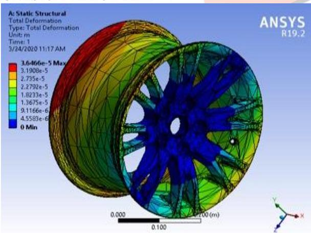
Figure 6. Total deformation of Mg-alloy RIM.
