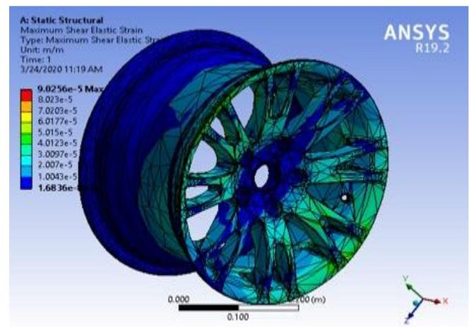
Figure 9. Maximum shear elastic strain of Mg-alloy RIM.
