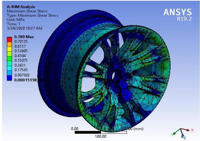
Figure 3. Maximum shear stress of Al-alloy RIM.
