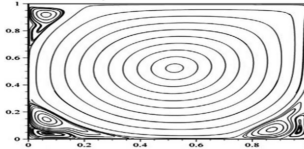
**Figure 01 :** Streamlines using EMMS turbulence model.
