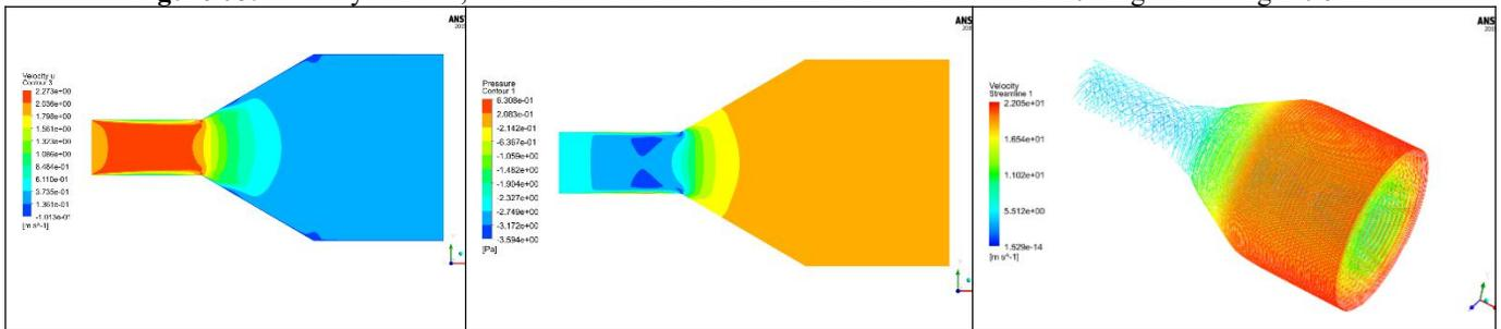
**Figure 09:** Velocity contour, Pressure contour and streamlines for diffuser with 30° angle and length 0.51m
