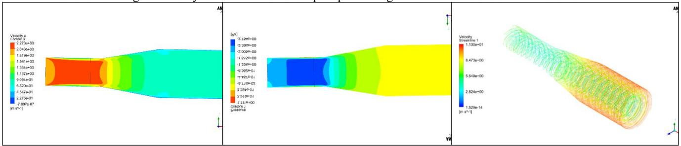
**Figure 07:** Velocity contour, Pressure contour and streamlines for diffuser with 10° angle and length 0.51m
