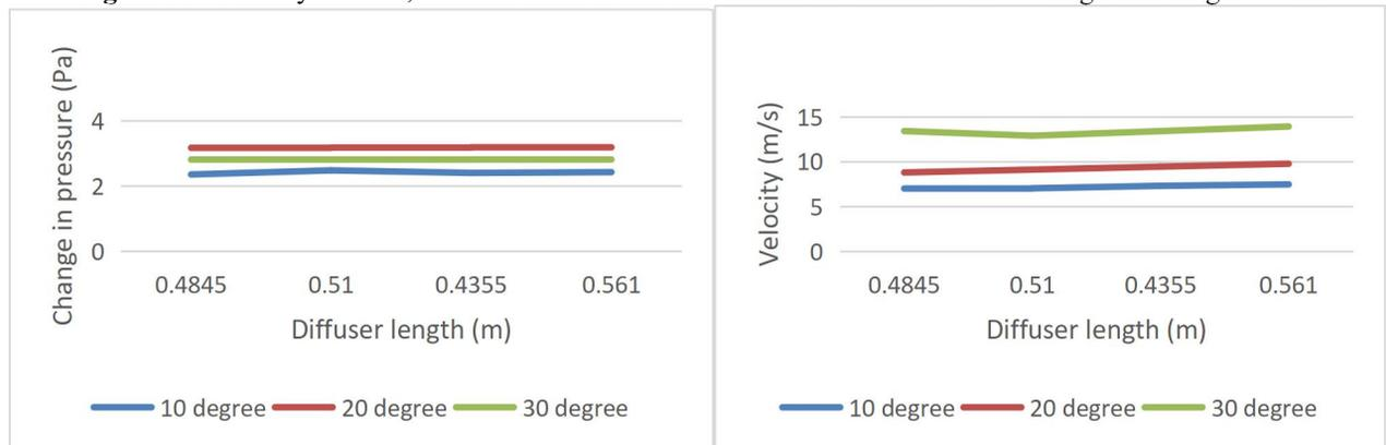
**Figure 10:** Chart of velocity and change in pressure w.r.t diffuser length for all cases
