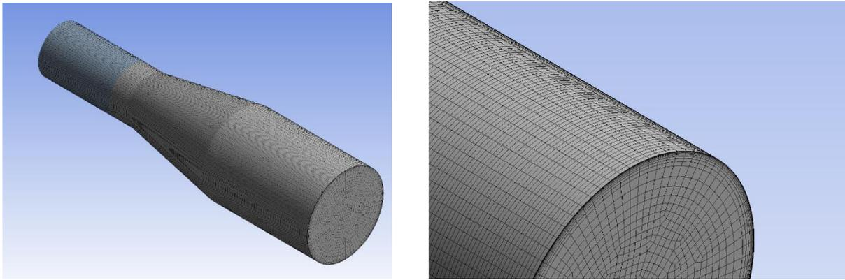
**Figure 04:** Meshing of CAD model isometric view and its zoomed view.
