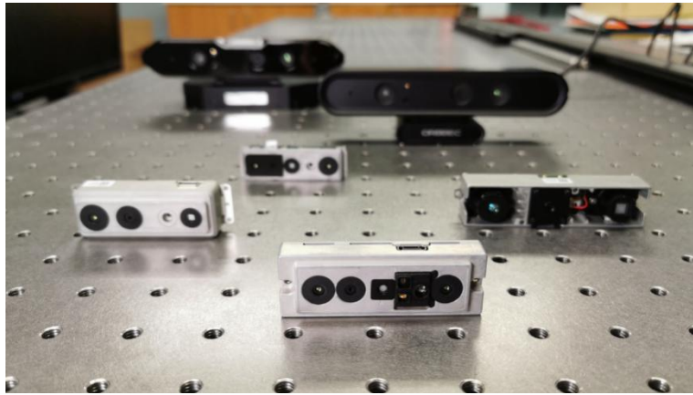
Figure 6: Orbbec's four basic models of its Astra series 3D camera, with some model-specific variations, and the Persee-model camera (back left).
