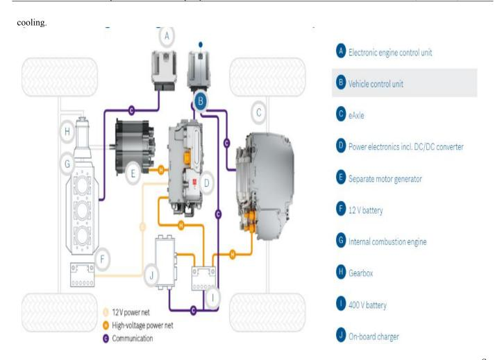
ystem map of an Electric Hybrid Vehicle can be seen here. The highlighted Marker B is the Vehicle Control Unit essentially serving as the brains of the Powertrain operation other excluding the IC engine marked by Marker G. [2]
