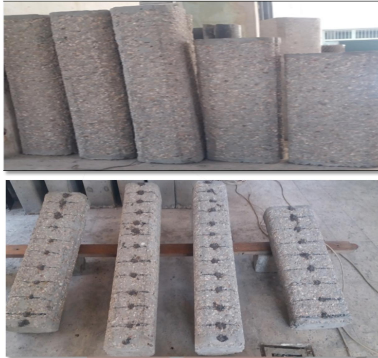
Fig5. The fixation of the nails at the column's surface.
