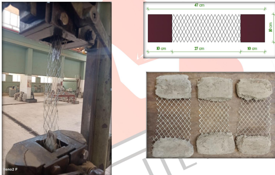
Fig 3. The specimens of the wire mesh and the tensile test
