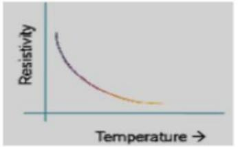
Figure 7: Variation of Resistivity with Temperature
