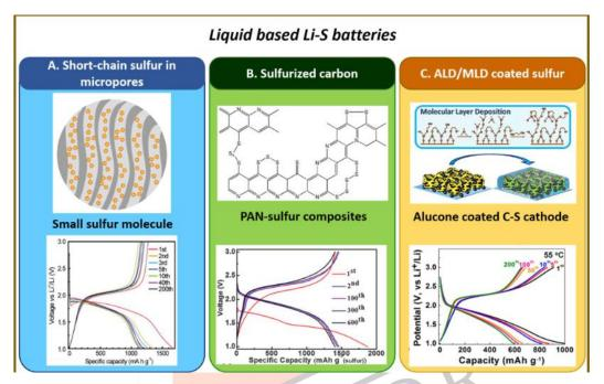
Figure 12 Different sulfur cathodes delivering solid-phase Li-S electrochemical reaction.
