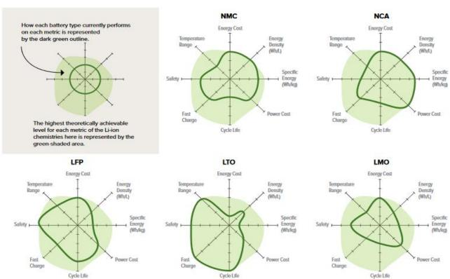
Figure 4 Selected performance of various Li-ion battery
