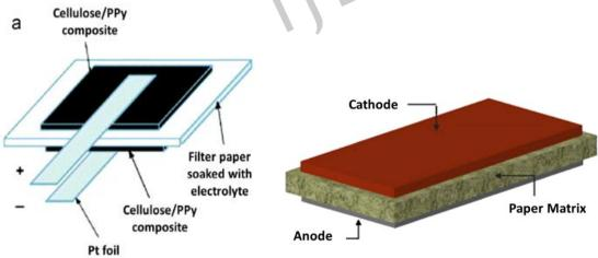
Figure 8 Schematic Diagram of paper battery
