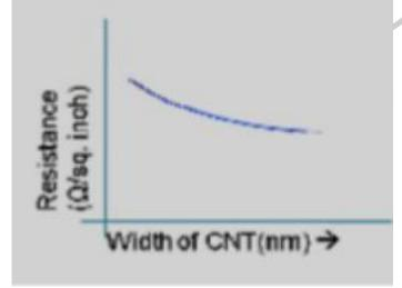
Figure 6: Variation of Resistance with Width of CNT
