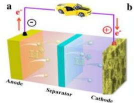
Figure 10. Schematic Diagram of Li-Sulfur Cell
