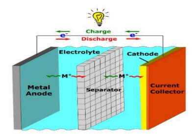
Figure 3. Battery with its components
