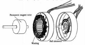
Fig 6. Disassembled view of BLDC motor
