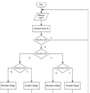
Fig 5. Perturb and Observe flowchart
