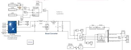
Fig 9. Model of BLDC motor with solar PV array
