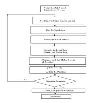
Fig 8. PSO Algorithm for tuning of BLDC Motor Controller
