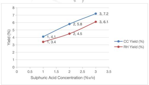
Fig. 1: Effect of Sulphuric Acid Concentration (% v/v) on Bioethanol Yield
