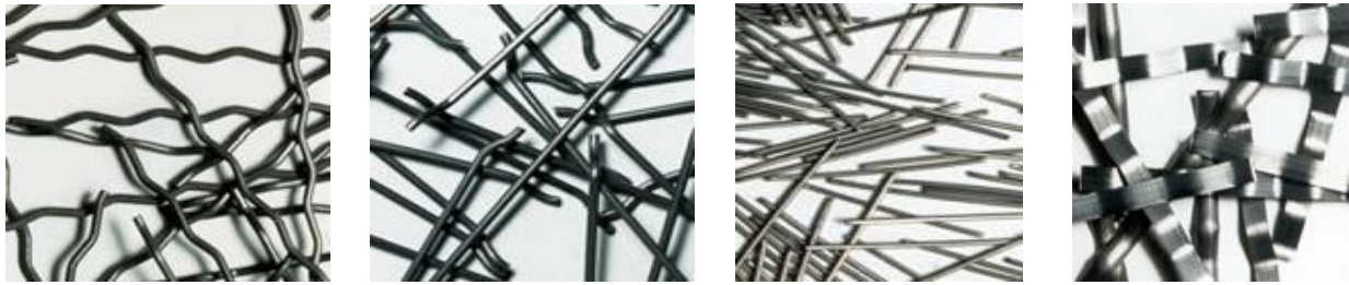
a) Undulated steel fibre b) Hooked end fibres c) Straight fibres d) Crimped steel fibres
