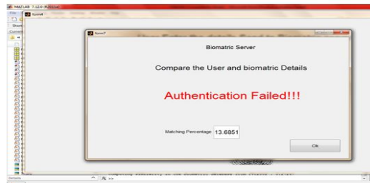
Fig.7 Fuzzy logic Compare the user finger print image and User is not authenticated by comparison result is below 60 %
