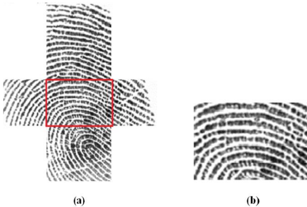
Fig.6 Compare both cropped image and extract common part. (a) Comparison of both cropped image based on vector values. (b) Extract common part.
