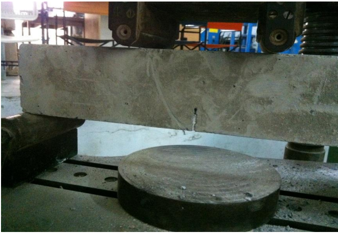
Fig 3. Flexural test on concrete beam
