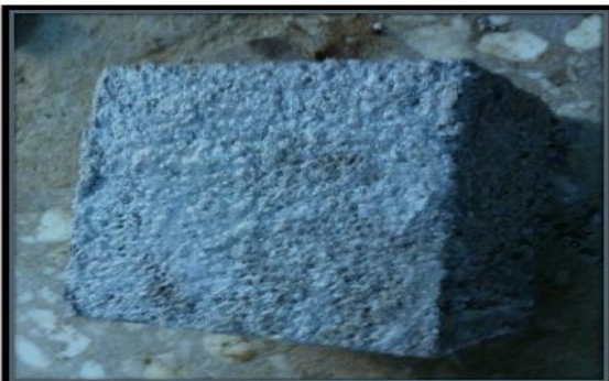
Fig. 4 – Cube After 28 day immersed in MgSo 4 Solution
