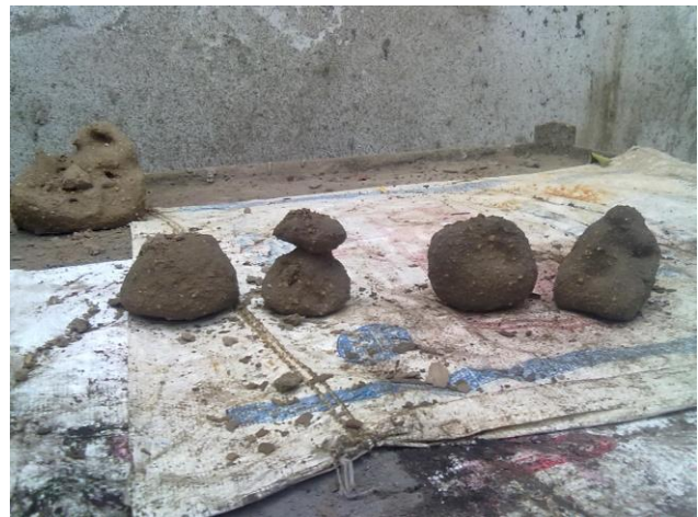
Figure -5 Deteriorate samples after Spray test
