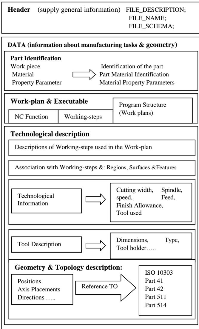
Figure 3- The general structure of a STEP compliant NC code [3].
