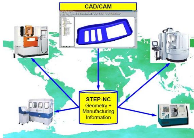
Figure 2. Tomorrow CAM and CNC[20]
