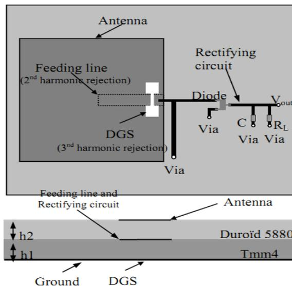
Figure 5: micro-strip antenna used for harmonic rejection
