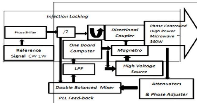
Figure 3: Block diagram of Phase Controlled Magnetron
