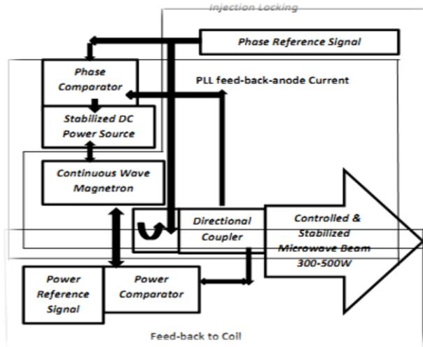
Figure 2: Block Diagram of PACM
