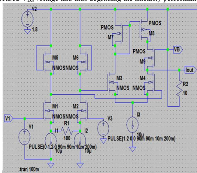
Figure9: The Design Architecture of Transconductor Cell
