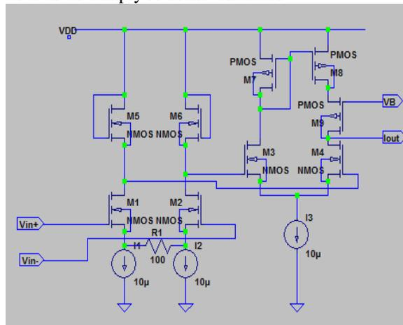
Figure1: The proposed transconductor cell
