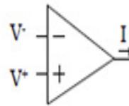
Figure 3: An Operational Transconductance Amplifier
