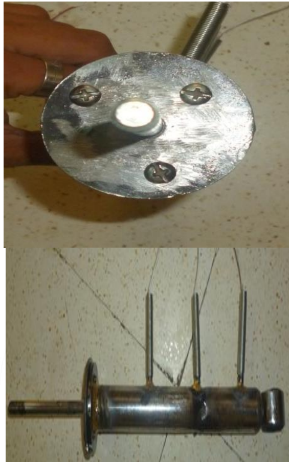
Fig. 3 Shock absorber modifications (www.ijesrd.org)
