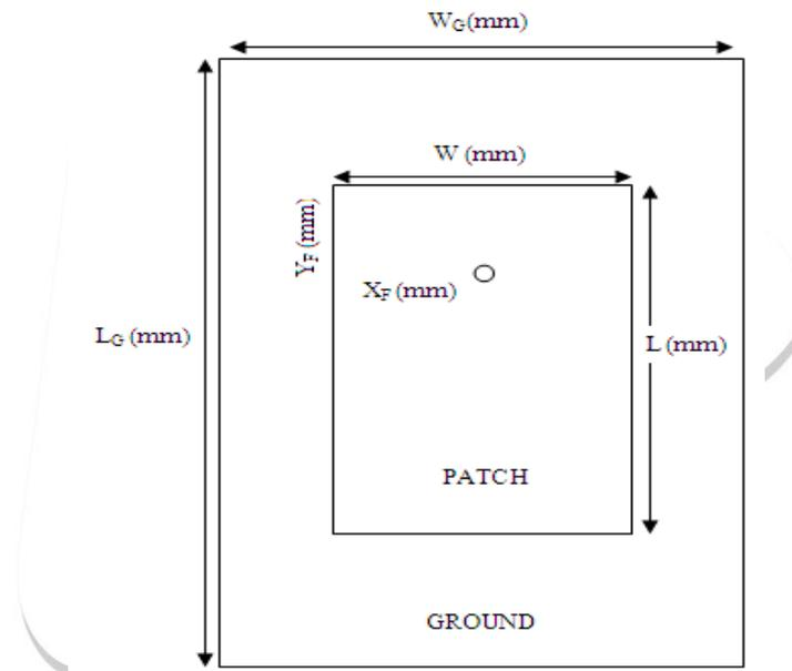
Fig.2. Schematic of the rectangular patch antenna
