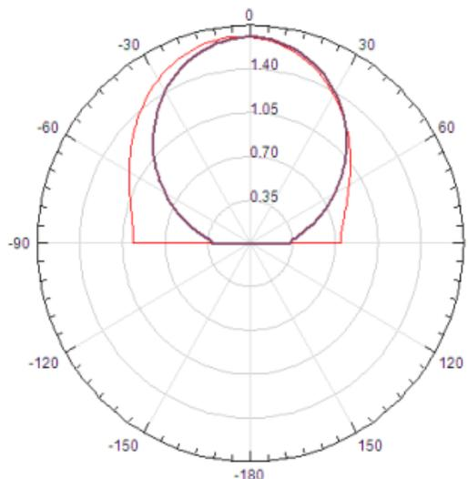
Fig.6. Radiation Pattern of the antenna
