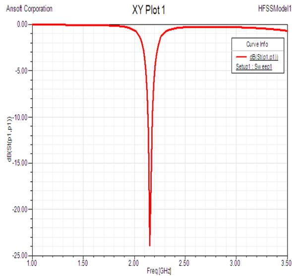
Fig.4. Return Loss of the antenna in HFSS (-22dB)
