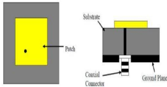
Fig.1. Co-ax fed patch antenna
