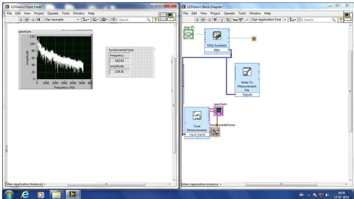
From the fig, it is seen that the experimental frequency of sound measured is about 183 Hz. From the amplitude versus frequency plot it is seen that the maximum amplitude is at the frequency about 183 Hz.
