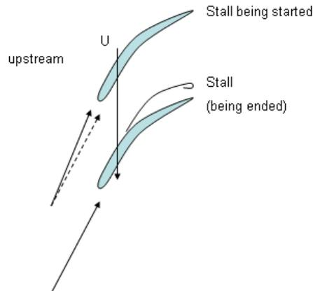
Repeatedly, the stall cell turns around the blades at about 30~50% of the running frequency and the direction is opposite to the blades. This series of phenomenon causes unsteady blade forces, and consequently generates noise and vibrations.
