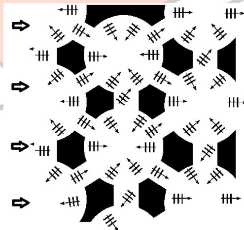
Highly porous materials are not suitable for acoustic absorption. If the mean free path of air is on the order of that of mean distance between pore walls, pressure wave will not be able to efficiently penetrate the material.
