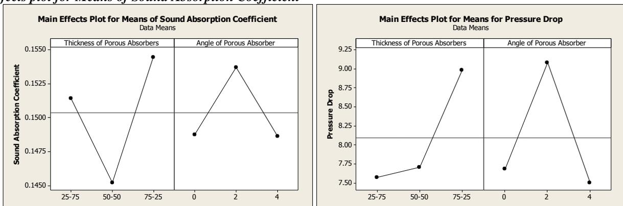
From the fig, for plot of Means of sound absorption coefficient, it is seen that for the third level of thickness i.e. 75 mm thickness of Elastomeric Foam and 25 mm thickness of Glass Wool and second level of angle i.e. 2° angle of the porous absorber the sound absorption coefficient is high.
