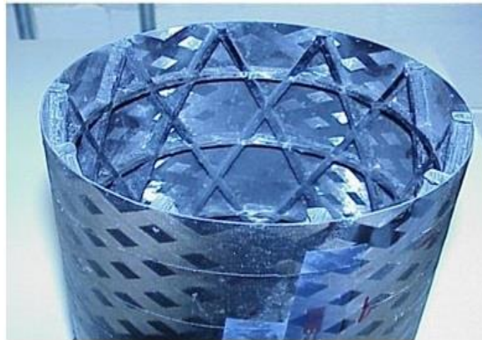
Fig: 7. Test specimen: isogrid stiffened composite cylinder.
