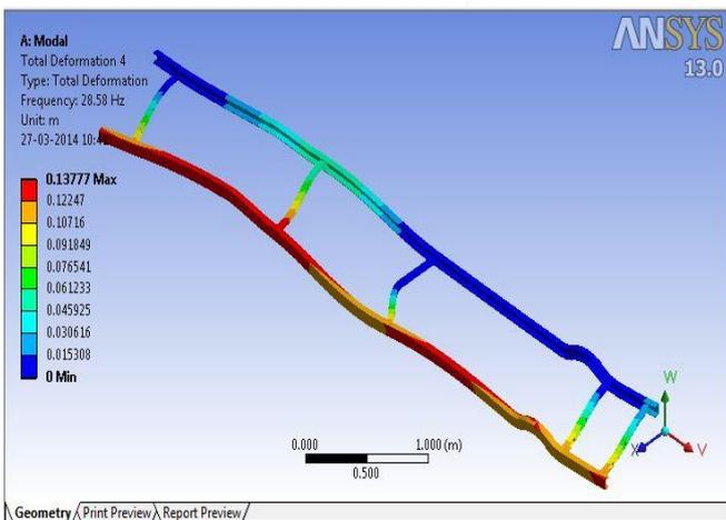
Fig 4.5 Deformation 4<sup>th</sup> Mode
