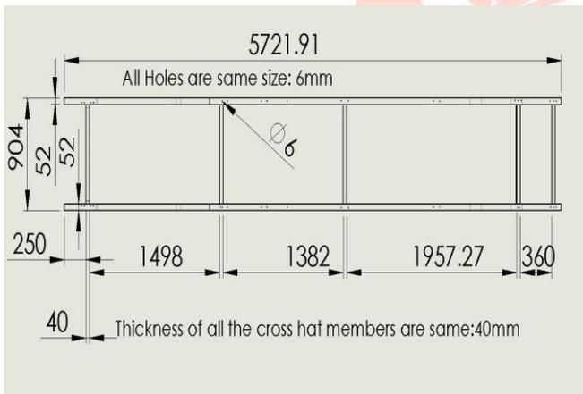
Fig 3.3: Top view of Chassis
