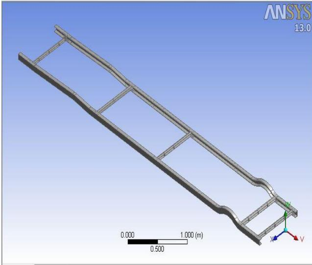
Fig 3.1: Geometric model of Chassis
