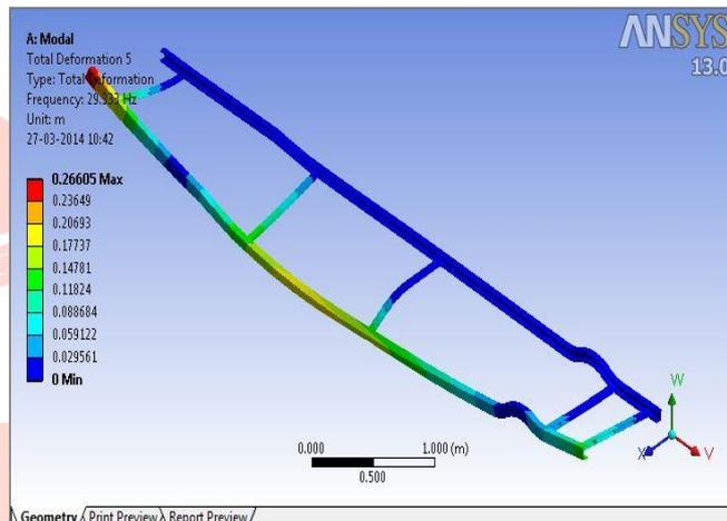
Fig 4.6 Deformation 5<sup>th</sup> Mode
