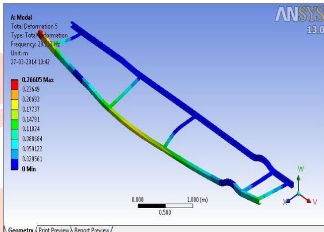
Fig 4.6 Deformation 5<sup>th</sup> Mode
