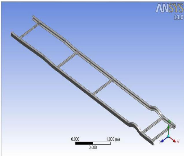
Fig 3.1: Geometric model of Chassis
