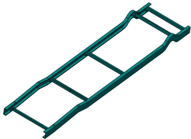
Fig 3.2: Truck Chassis Frame Along With Cross Members
