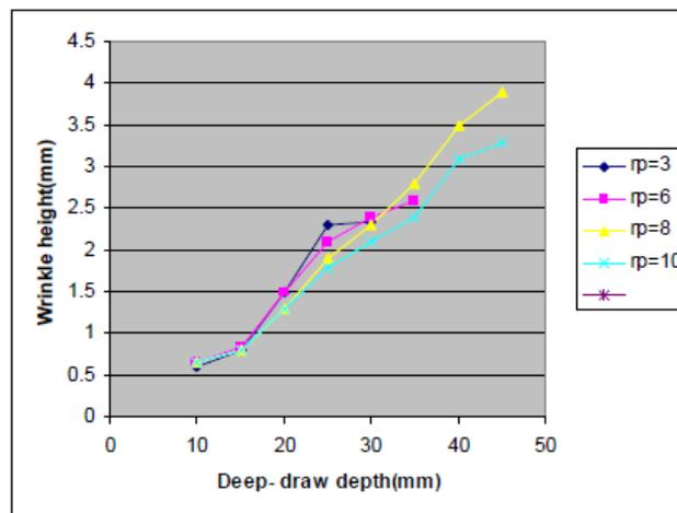
Fig. 4 The Influence of the Die and Punch Edge Radius on the Wrinkling
