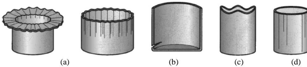
Fig. 2 Various Defects in Deep Drawing Process [2]
