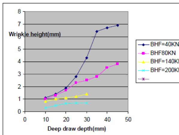
Fig. 3 The Effect of the Blank Holding Force and the Deep Drawing Depth on the Wrinkling
