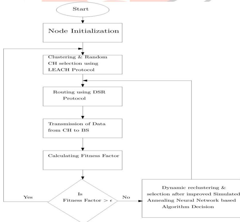
Fig 2: Proposed algorithm of Improved Neural Network based Dynamic Clustering in WSN
