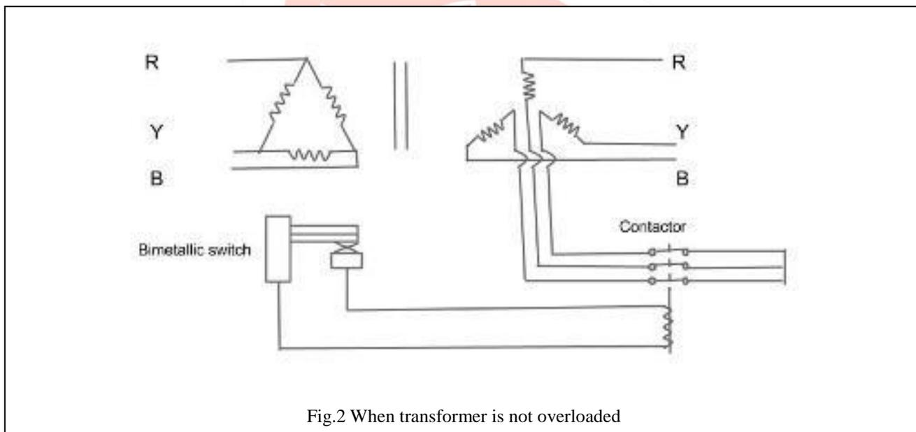
If again the temperature of the transformer is increased the bimetallic switch will change the state and contactor will open the connection of the secondary of the transformer and transformer will stop the working. this process is done according the temperature of the transformer.
