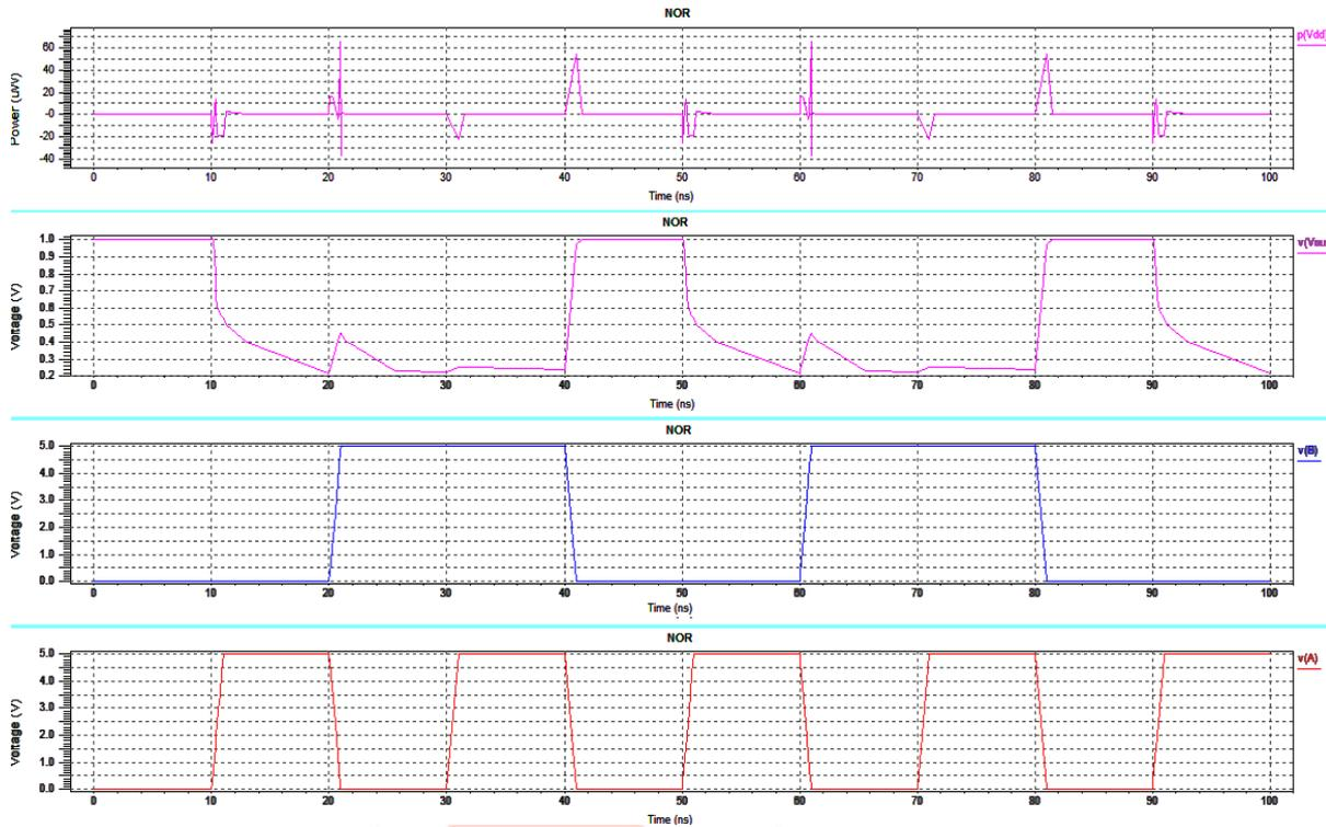
Figure.8:Simulation waveforms of LCnMOS NOR gate
