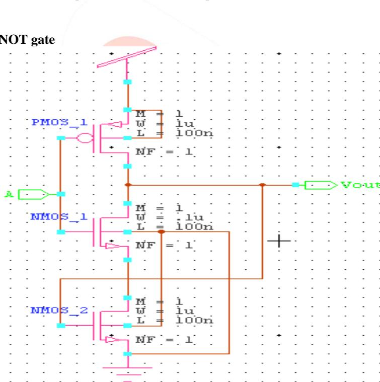
Figure 3. LC nMOS based NOT gate
