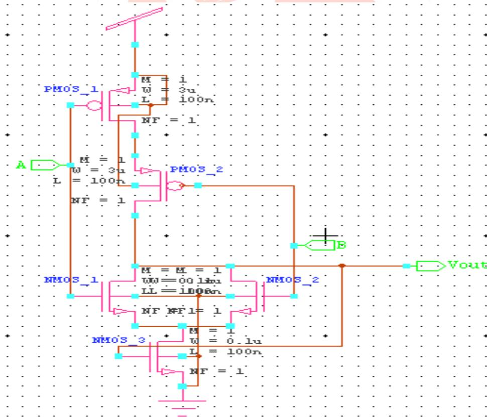
Figure.7:2-Input LCNMOS NOR gate
