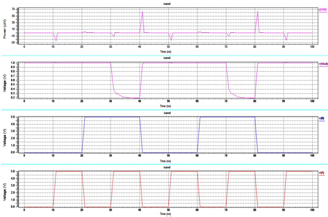
Figure.6:Simulation waveforms of LCNMOS NAND gate
