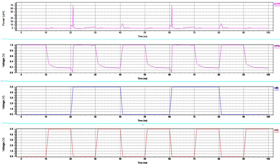
Figure 4 Simulation Waveform of LCnMOS Inverter
