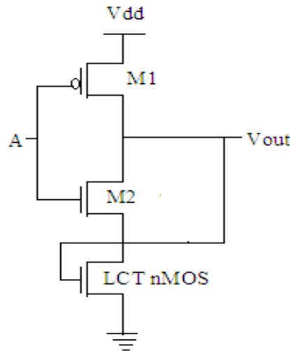
Figure 2. LC nMOS based CMOS Inverter
