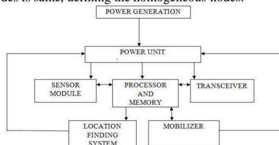
**Fig.1. Components of sensor node**
