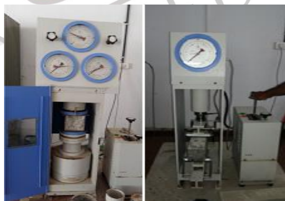
Fig. 2 Test setup for compressive strength and flexural strength
