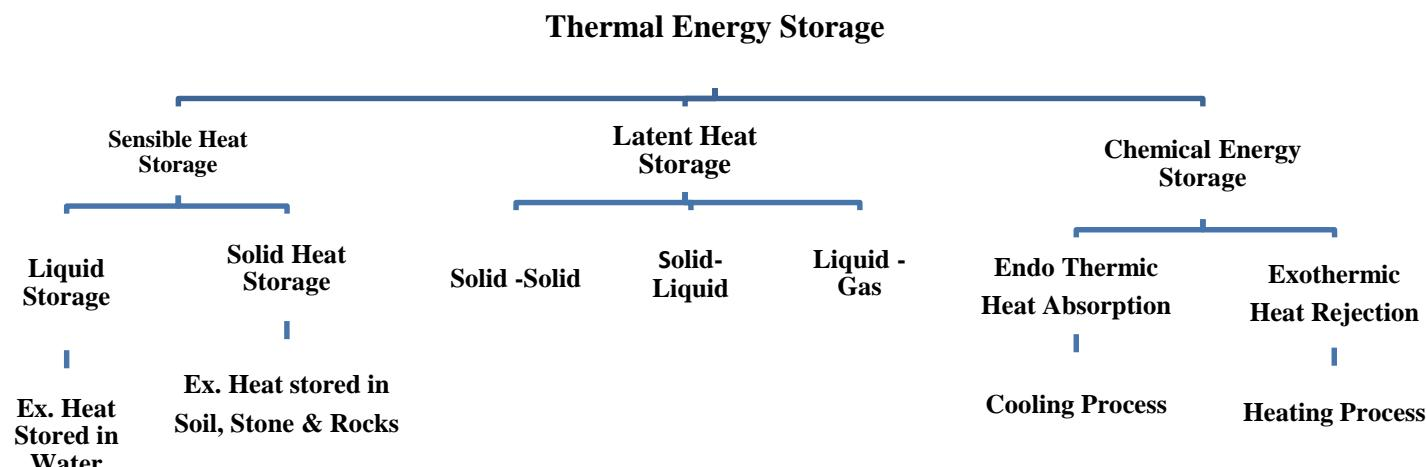
In this present review work various methods of storing thermal energy storage in different materials and different systems.
