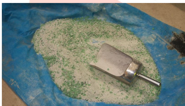
Fig 3: Glass waste crushed through abrasion machine
