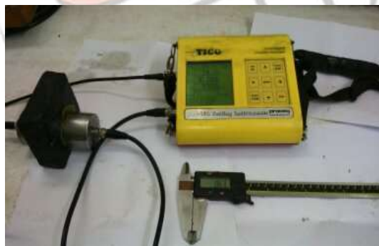
Fig (2) Experimental Set-up for Velocity Measurement
