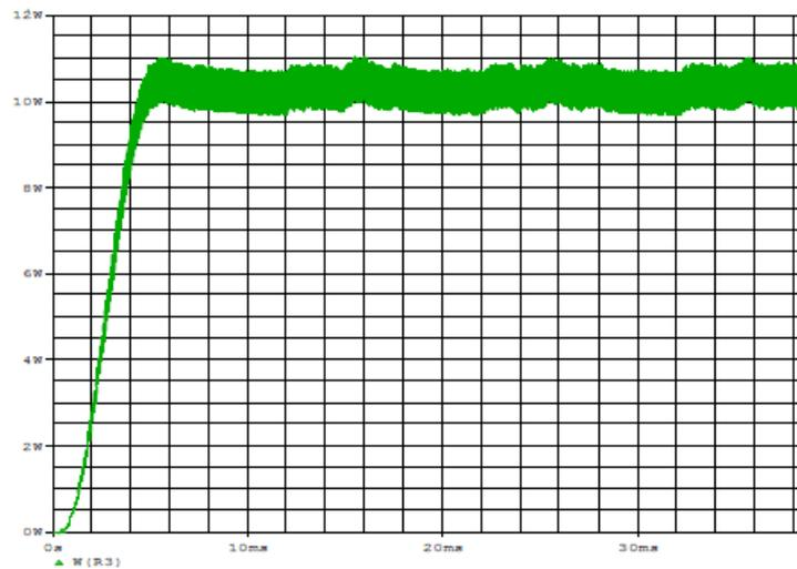
**Figure 16:** Output power with for a case of voltage ripple less than 5%.
