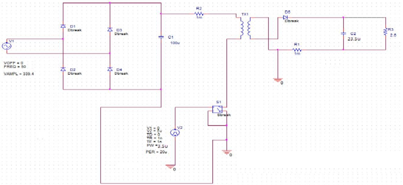
**Figure 1:** Simulated circuit of iPad cell charger
