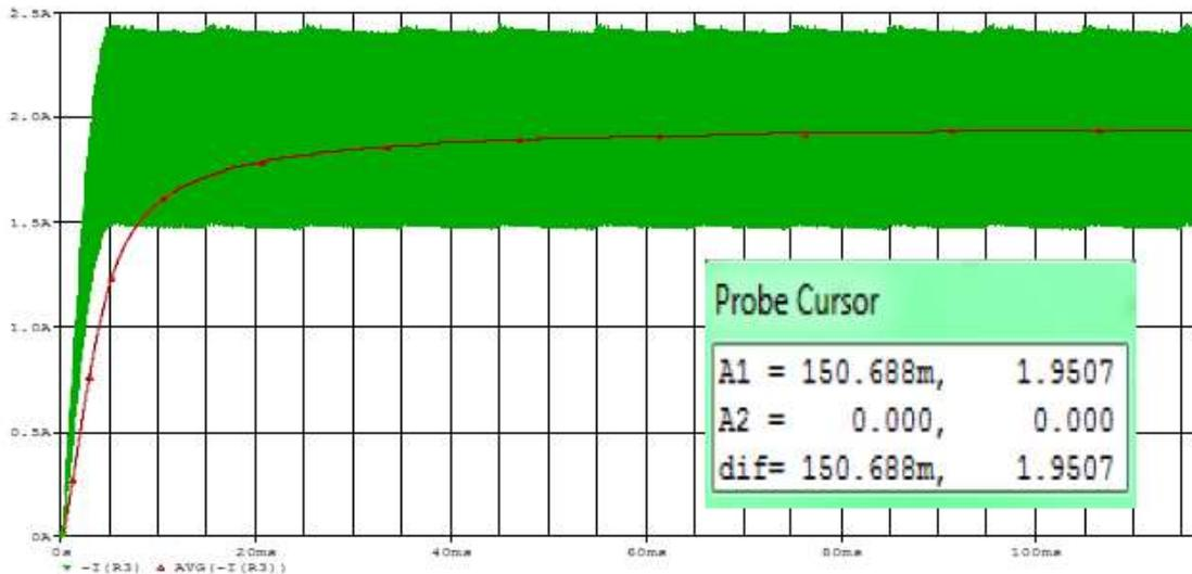
Figure 11: Output Current after using the new values for PW, D and C.
