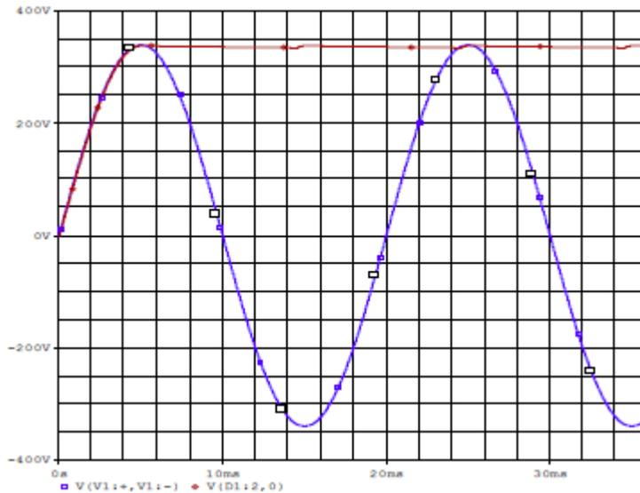
**Figure 2:** Input Voltage (blue) and Output Voltage (red) of Rectifier (C<sub>1</sub>)
