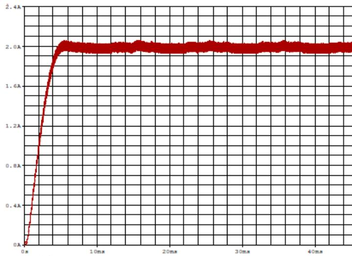
**Figure 15:** Output Current with for a case of voltage ripple less than 5%.
