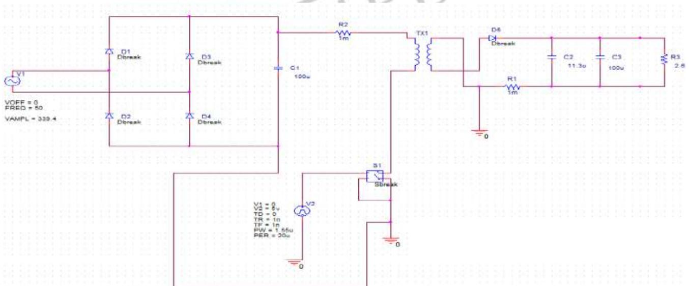
Figure 13: Simulated circuit of cell charger with voltage ripple less than 5%.
