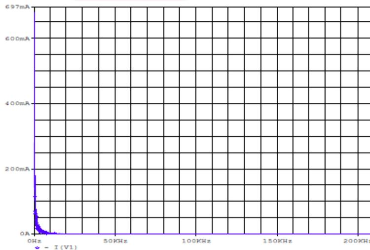
**Figure 4: Fourier Series of the Input Current (mA)**
