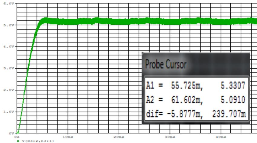
**Figure 14:** Output Voltage with voltage ripple less than 5%.
